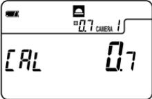
3. The calibration setting can be changed by rotating the Jog wheel while pressing and holding down the ISO 1 and ISO 2 buttons simultaneously. A range of +/- 1.0 EV in 1/10 step increments is possible for calibration.
