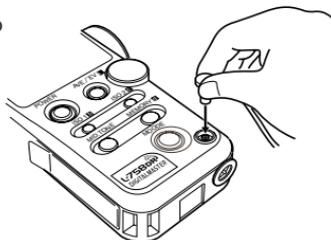
2. Hold down the Mode button and turn the Jog wheel to select cord flash mode ⑬.
