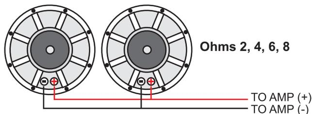
If using SINGLE 2 OHM coils the total load would be 1.0 ohm
