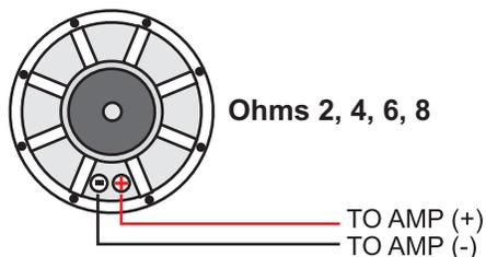
If using SINGLE 2 OHM coils the total load would be 2.0 ohm
