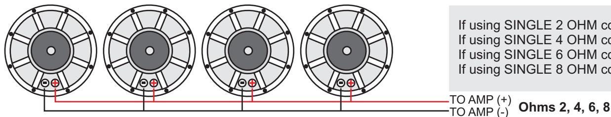
If using SINGLE 2 OHM coils the total load would be 0.5 ohm
