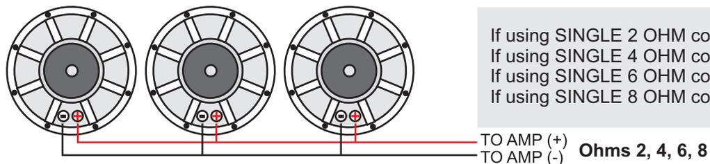
If using SINGLE 2 OHM coils the total load would be .66 ohm
