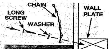
4. Attach the stability chain so that it lines up with the bracket on the back of the range.
