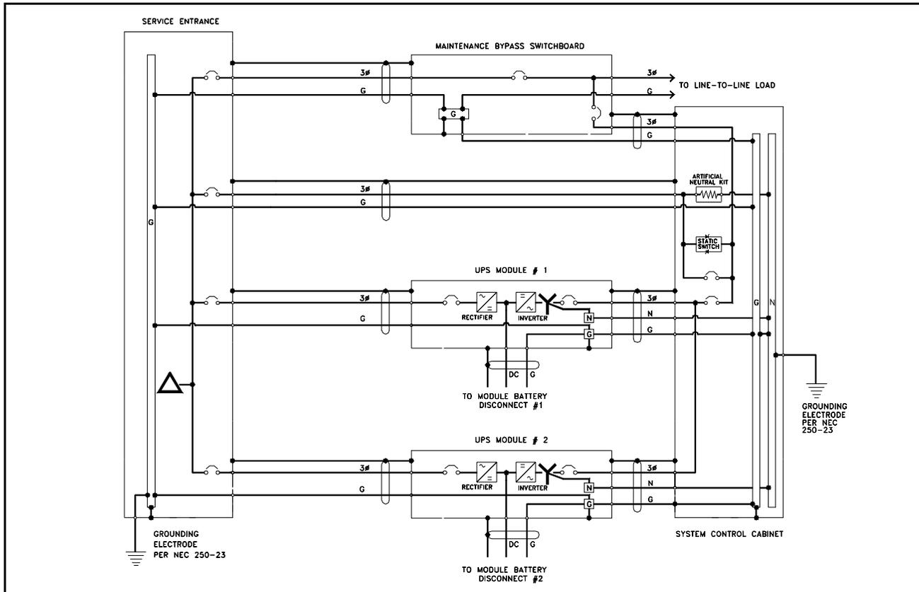
As previously mentioned, Series 600T UPS systems require a bypass input neutral for sensing and monitoring. With a wye-connected input source, the installer should always connect the building service neutral to the System Control Cabinet (SCC) output neutral to achieve this. When the building service is delta-connected, however, the installer must take special steps to ensure reliable UPS functioning.
