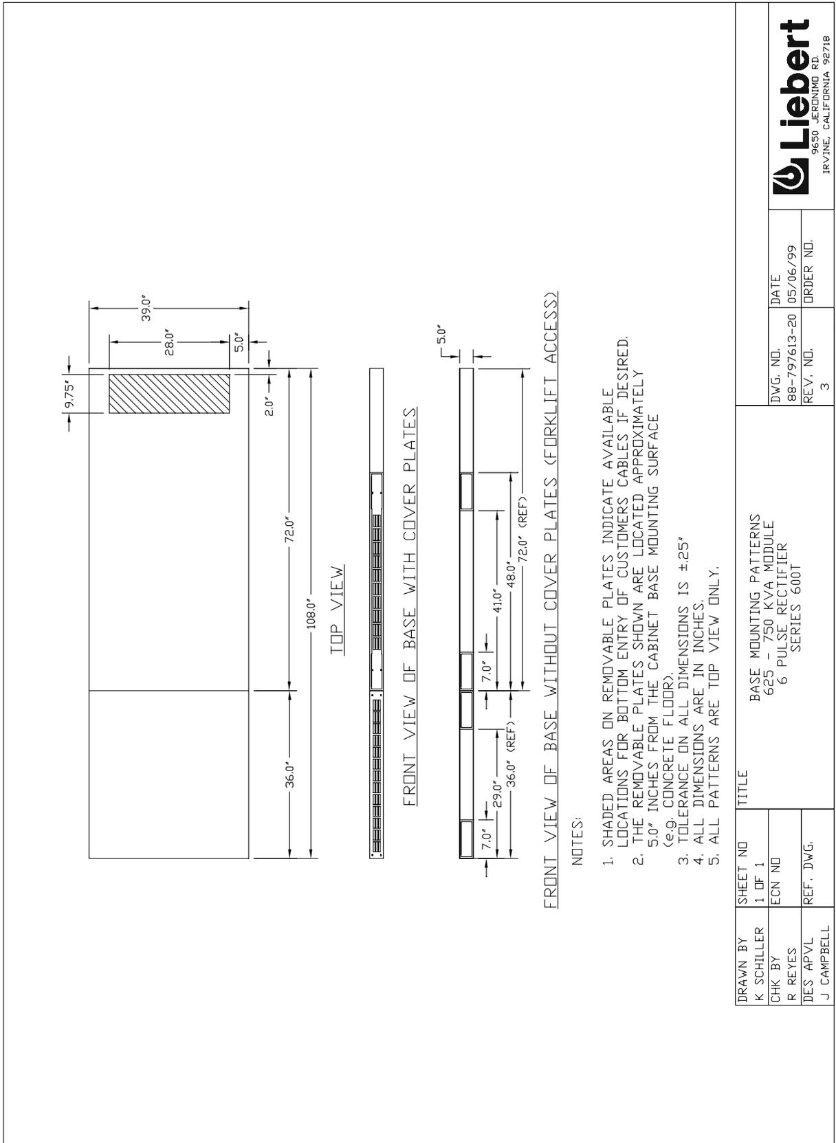
Figure 21 Base Mounting Patterns, 625-750 kVA Module, 12-Pulse Rectifier
