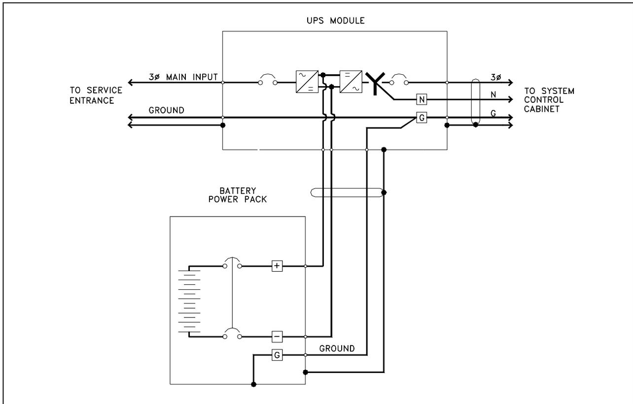
Large, open-rack battery systems are normally either locally grounded or left ungrounded, depending on local code requirements.
