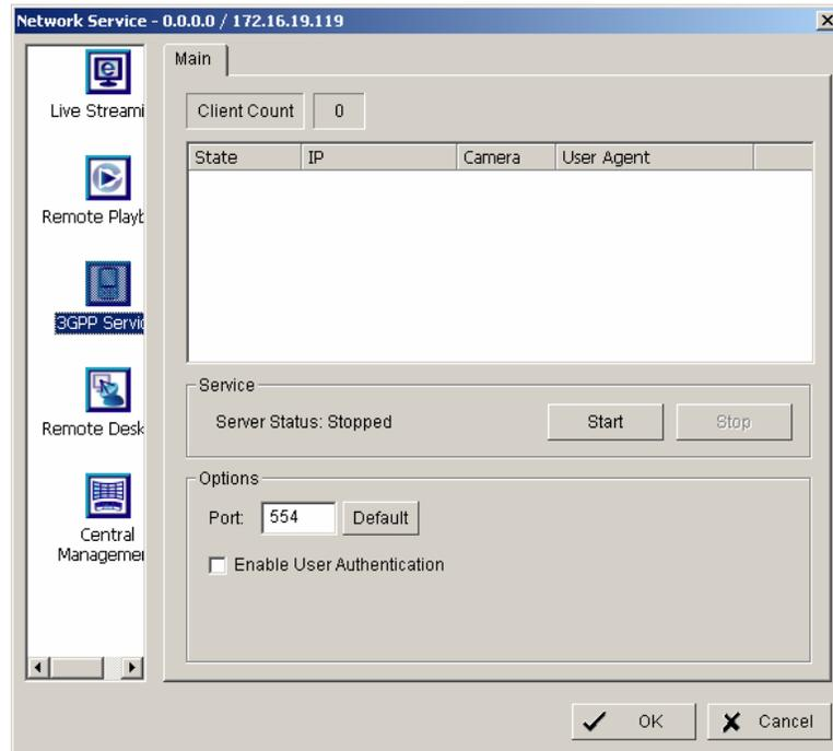
**Service Start / Stop** By clicking on START the server function for 3GPP service is enabled.
