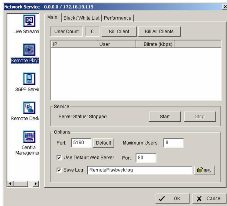
**Service Start / Stop** By clicking on START the server function for playback view is enabled.
