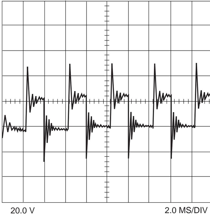
This is a typical DC output voltage waveform generated from a properly operating machine. Note that each vertical division represents 20 volts and that each horizontal division represents 2.00 milliseconds in time.
