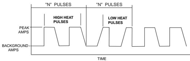
The Peak Current, Background Current, and Frequency are identical for the high energy and low energy pulses. In addition to cooling the weld down, the major effect of the low energy pulses is that they form a weld ripple. Since they occur at very regular time intervals, the weld bead obtained is very uniform with a very consistent ripple pattern. In fact, the bead has its best appearance if no oscillation of the welding gun ("whipping") is used. (See Figure B.7)
