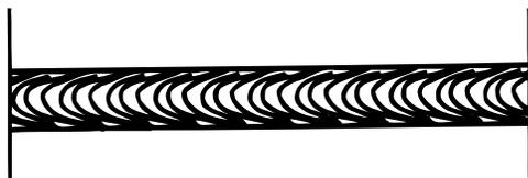
When Arc Control is used in the Pulse on Pulse modes, it does the same things it does in the other pulsed modes: decreasing the Arc Control decreases the droplet transfer and weld deposition rate. Increasing the Arc Control increases the droplet transfer and weld deposition rate. Since Arc Control varies weld droplet transfer rate, the Arc Control can be used to vary the ripple spacing in the weld bead.
