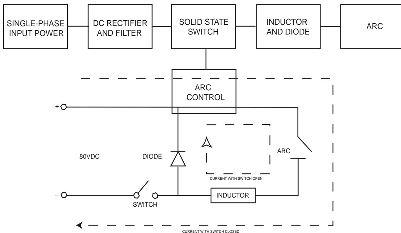
In this system, the engine drives a three-phase alternator, which generates power that is rectified and filtered to produce about 80VDC. The current is applied through a solid state switch to an inductor. By turning the switch on and off, current in the inductor and the arc can be controlled. The above diagram depicts the current flow in the system when the switch is open and closed:
