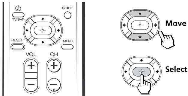
To navigate on the on-screen menu, use the “arrow” buttons (↑, ↓, ←, →) to move the cursor. Pressing these arrows will cause the cursor to move in the corresponding direction. Pressing center button (⊕) will allow you to select an option.
