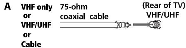
Use this to connect the TV to a cable system or an antenna with a 75-ohm cable (usually built into newer homes).
