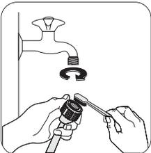
Turn off the water tap. Unscrew the water inlet hose. Clean the filter using a hard bristle brush.
