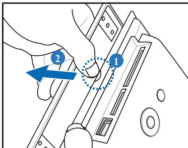
3. To install a new front panel, align the panel edge to the Digital Photo Frame and gently place the panel on the device.
