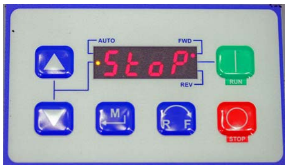
Figure 15 VFD Control Panel
