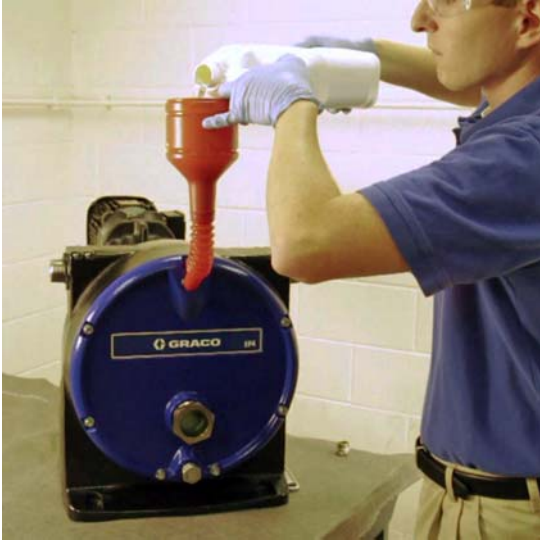
Figure 4 Fill Pump With Hose Lube
