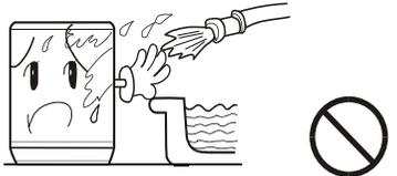
Do not wash water-proof laundries like the raincoat, bike covers etc. to avoid abnormal vibrations in spinning.
