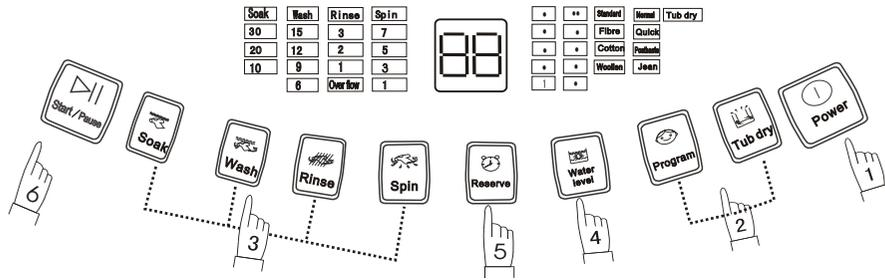
1. Push "power" button to switch on the power
