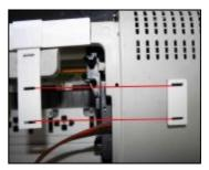
Fix the balance arm stick on the support arm as show on the picture, Rip the label on the shortest arm ,And Stick it on the right side of the printer, but need to keep it in the same horizontal line as show in the picture
