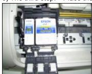
Remove out the original cartridges
