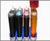
Please pay attention to the ink level in the reservoirs; if the ink level is below 1CM as the above picture shown, please use refill kits to fill ink into Reservoir bottles. Carefully pull out the rubber plugs from the refill holes.(there is possibility of ink spattering. Be careful!) Refill ink according to the color in short supply. Then put the rubber back. (Please keep the printer and the reservoir at the same horizontal line during the process of refilling ink.)
