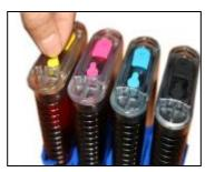
Remove from the air hole as above picture shown.
