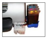
Put the CISS on the right side of the printer. In the meantime place all the tubes at correct position.
