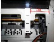
Stick the Support arm at 7.5cm distance from the inner side of the printer, Rip the
