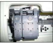
to make the small cart button move to the position which ready to change the ink cartridges
