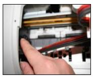
Adjust the tube length and move the cartridge car. Insure there will no block and collision when the tubes moving with cartridge car .Insure there's plenty length of tube to make the cartridge cart can thoroughly move to the right side.
