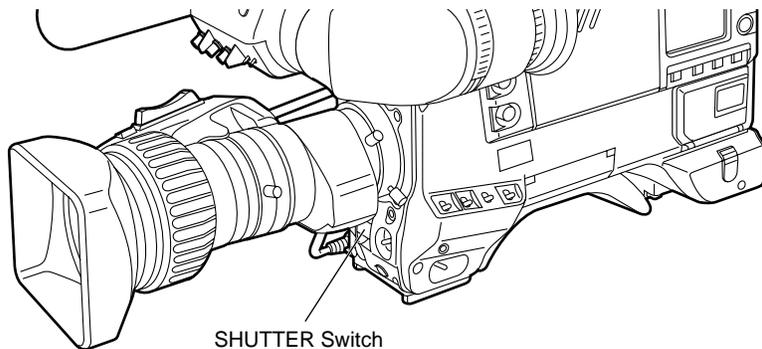
**3** Press the SHUTTER switch to the SEL side repeatedly until the desired mode or speed appears. When all modes and speeds can be displayed, the display changes in the order shown below. If the required shutter speeds and modes have been designated beforehand, only the designated speeds or modes appear.
