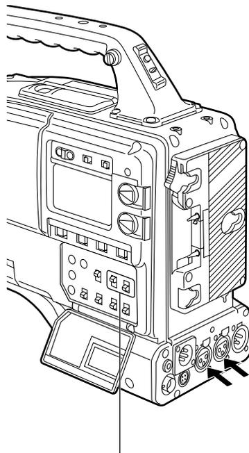
Up to two external microphones can be connected to the AUDIO IN CH1/CH2 Connectors. Phantom power supply can also be supported by setting the MIC POWER switch to the ON position.
