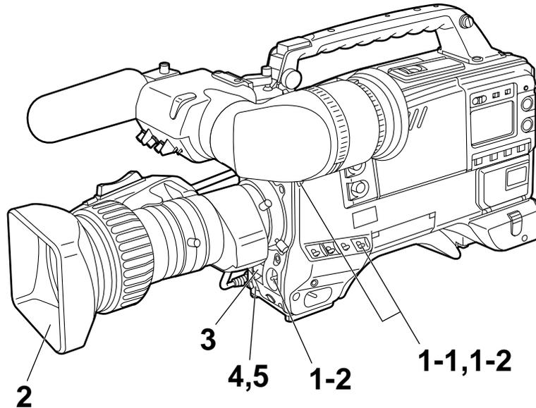
**1-1** Select the filter in accordance with the lighting conditions, and when the white balance has already been stored in the memory, set the WHITE BAL switch to “A” or “B”.
