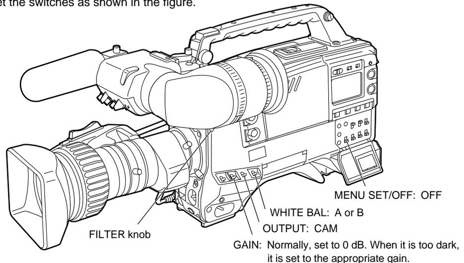
When the positions of the GAIN and WHITE BAL switches are changed, a message informing the operator of the new settings will appear on the setting change message display area of the viewfinder screen. (However, this display appears only when the display mode is set to “3”.)
