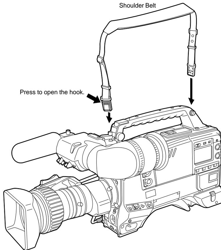
To remove the shoulder belt, open the hooks and then remove the belt.
