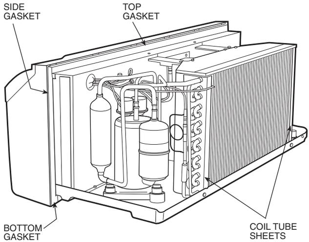
**FIGURE 8 — UNIT GASKETS AND TUBE SHEETS**
