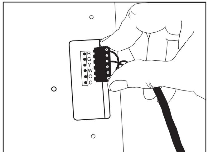
FIGURE 12 — TERMINAL CONNECTOR REMOVAL AND REPLACEMENT
