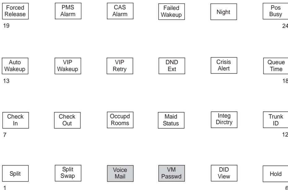
**Figure 24. Console Buttons with Voice Messaging**
