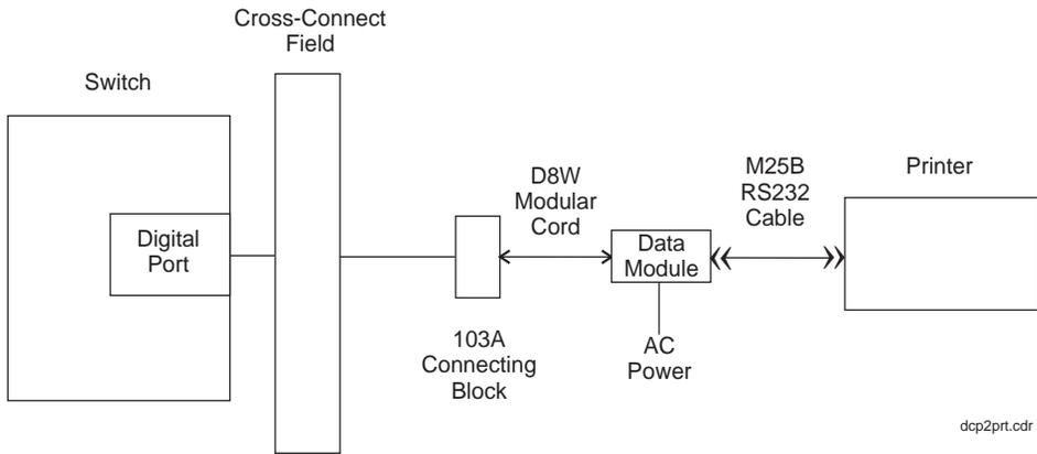
Figure 19. Printer Connections Using a Data Module
