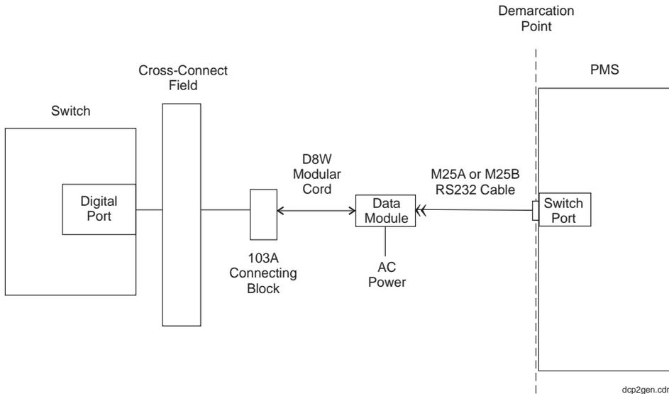
Figure 18. PMS Link Using a Data Module
