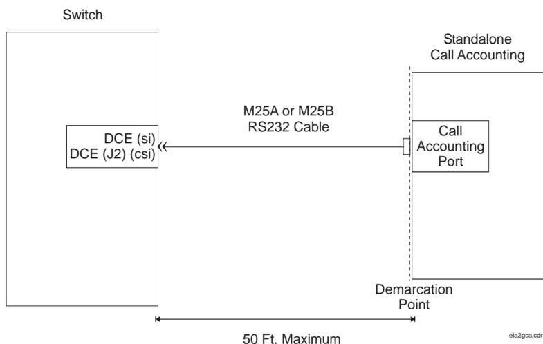
Figure 14. Switch-to-Call Accounting Link (Stand-Alone Call Accounting System)
