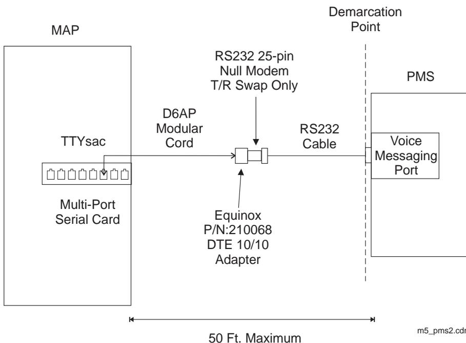
Figure 10. INTUITY Lodging-to-PMS Link (Multi-Port Serial Card)
