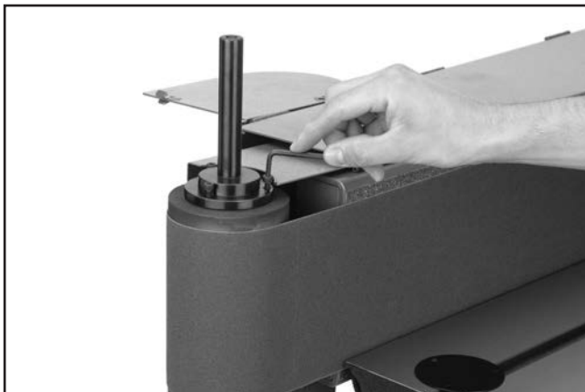
Figure 19. Tightening cap screws.
