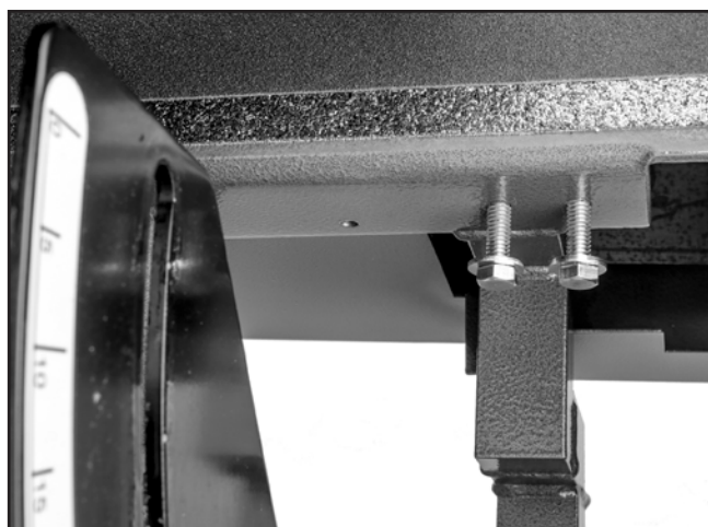
Figure 5. Back stop bolts.
