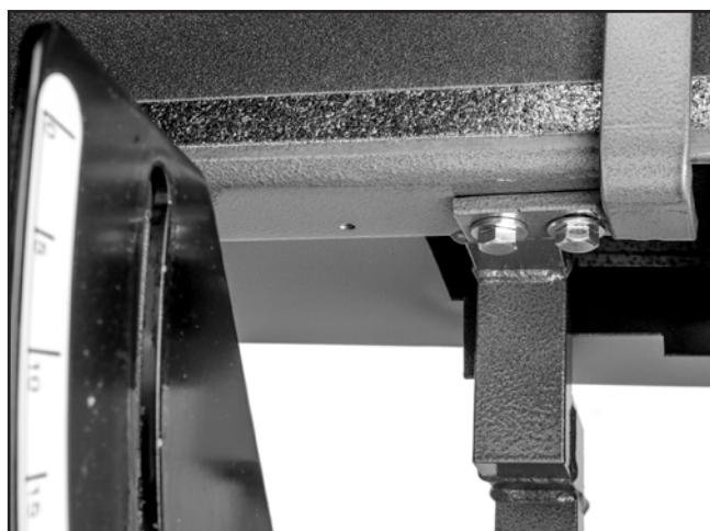
Figure 6. Back stop installed.
