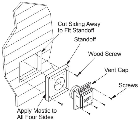
**Figure 11 - Installing Siding Standoff (Combustible Exterior Wall Only)**
