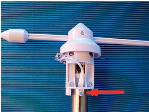
3. Insert the foot into the pipe and rotate it in such a way that it can be locked in the respective holes in the pipe using the two screws
