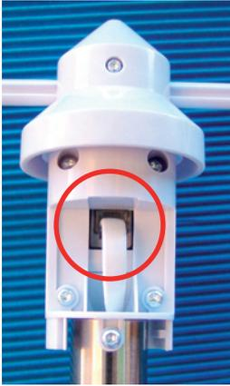
4. Insert the plug into the socket of the wind meter
