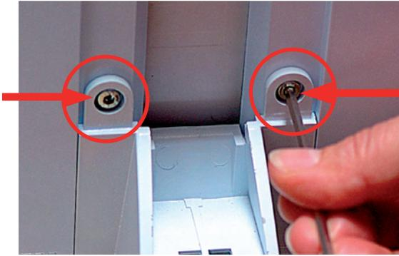
5. Screw the foot support on to the weather station using the enclosed Allen key and 2 Allen screws.
