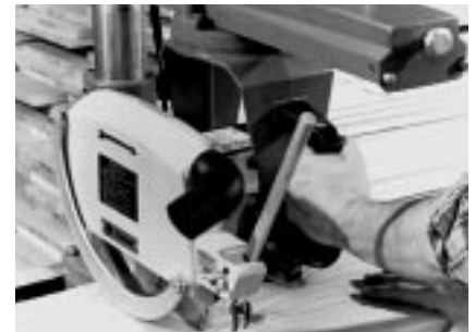
Powerful Motor with Mechanical Brake. 2 HP motor develops up to 4 HP peak under heavy workloads. Mechanical brake that's built into motor, stops blade automatically in seconds, after switch is turned off. This eliminates excessive blade coasting enabling production schedules to be maintained.
