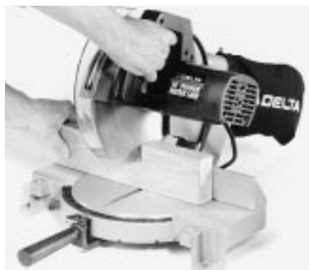
Crosscuts a nominal 2 x 6 or 4 x 4 at 90°. Miter a 2 x 4 flat or on edge in a single pass, at 45°.
