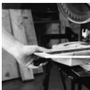
Quick-action miter lock eliminates use of traditional screw locks for faster miter setting.
