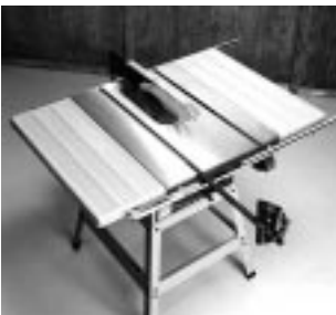
Cast iron 20" x 27" table with T-slotted miter gage grooves and two extension wings.
