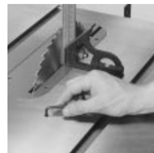
Unique "table top located" adjusting screws for accurate setting of 45° and 90° positive blade stops.
