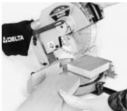
13 amp., 5200 rpm motor provides plenty of power and speed for tough cutting jobs.
