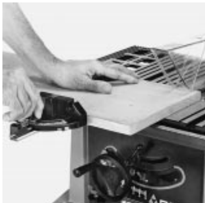
T-slot table groove prevents miter gage from falling during wide cut-off operations.
