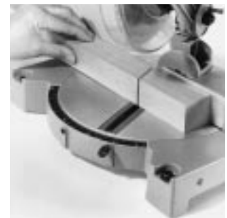
Positive detents on table facilitate miter cutting.
