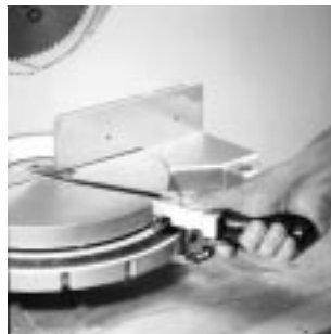
Patented trigger-controlled miter indexing mechanism facilitates quick, easy and accurate selection of 0°, 22½° and 45° R & L miter settings.
