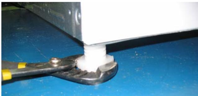
Press down on alternate corners and sides and feel for the slightest movement. Adjust the appropriate leg so the washer is SOLID on the floor on ALL four legs. Keep the leveling leg extension at a minimum for best performance of the washer.
