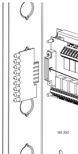
**NOTE:** *The LED display board is polarized and will only fit in one direction as shown. It must be fully inserted in order for the controller to function properly.*
