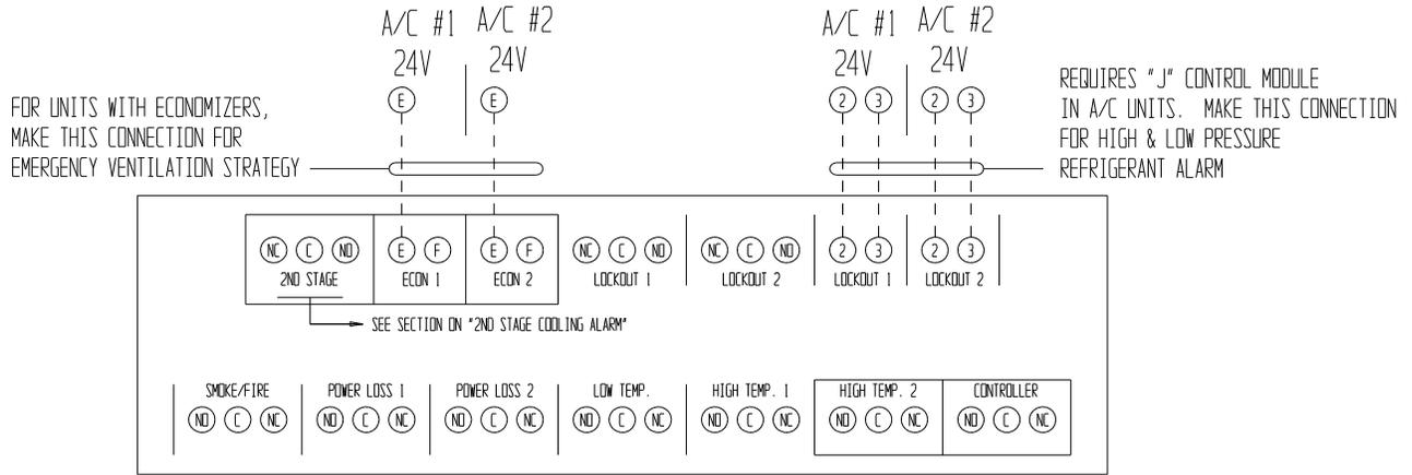
USE SHADED ○ TERMINALS FOR DESIGNATED ALARMS AS DESIRED. SOME RELAYS ARE REVERSE ACTIVATED TO ACHIEVE "NO" CLOSE-ON-ALARM SEQUENCE. EACH CAN BE USED INDIVIDUALLY IF THERE ARE ENOUGH BUILDING ALARM POINTS AVAILABLE OR CAN BE ARRANGED INTO SMALLER GROUPS OR EVEN A SINGLE GROUP SO THAT ALL ALARM CAPABILITIES CAN BE UTILIZED. FOR "NO" CLOSE-ON-ALARM STRATEGY MULTIPLE ALARMS IN A GROUP ARE WIRED IN PARALLEL.
