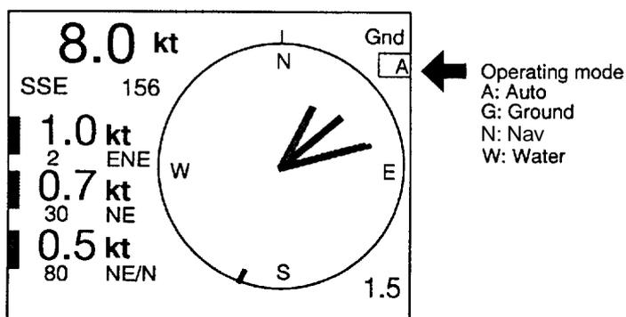
Figure 21 Location of operating mode indication on echo display
