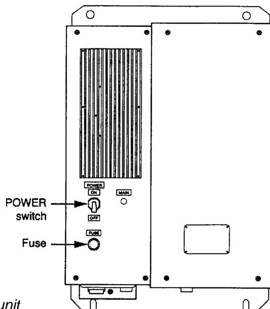
Figure 12 Transceiver unit
