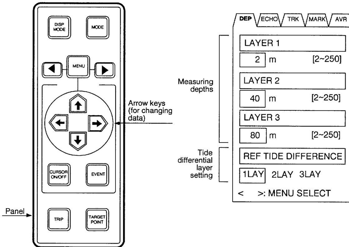
Figure 22 How to set tide differential
