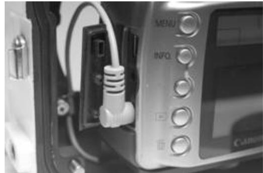
**Picture B: Trigger release cable position**
