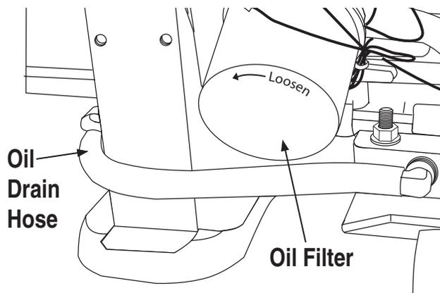
3. After the oil has drained, replace the cap onto the end of the oil drain hose. Retain the hose in the clip.
