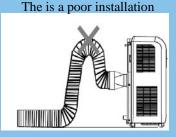
When installing the exhaust hose, try and keep it as flat as possible. The less angles and bends in the hose, the better the unit will perform. If bending or an angle is necessary, use single 90° angles like the pictures above. Multiple bends will decrease performance and efficiency
