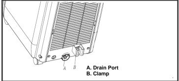
3) Attach the Drain Hose to the Drain Port using the Drain Hose Clip. Insert the Drain Plug into the free end of the Drain Hose and guide the Drain Hose through the Clamp. Once finished, the unit can be easily drained by removing the drain plug and guiding the drain hose into a small pan to drain the water.
