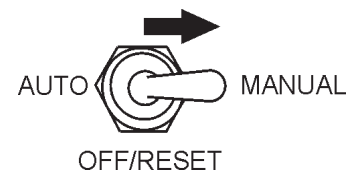
Figure 42. MPEC Control Switch (Manual Position)
