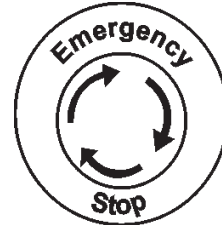
Figure 58. Emergency Stop Button
