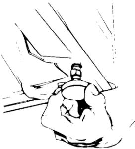
**14.** Tilt washer backward and remove corner post(s). Gently lower washer to floor.
