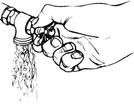
**9.** Before attaching water inlet hose, run water through both faucets into a bucket. This will get rid of particles in the water lines that might clog hoses. Mark which is the hot water faucet.
