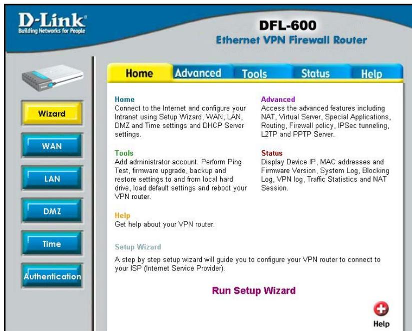
The Setup Wizard will guide you the most basic setup tasks, such as setting an administrative password, selecting the type of WAN connection you have, entering your computer's host name (if required by your ISP), saving the configuration and restarting the router.
