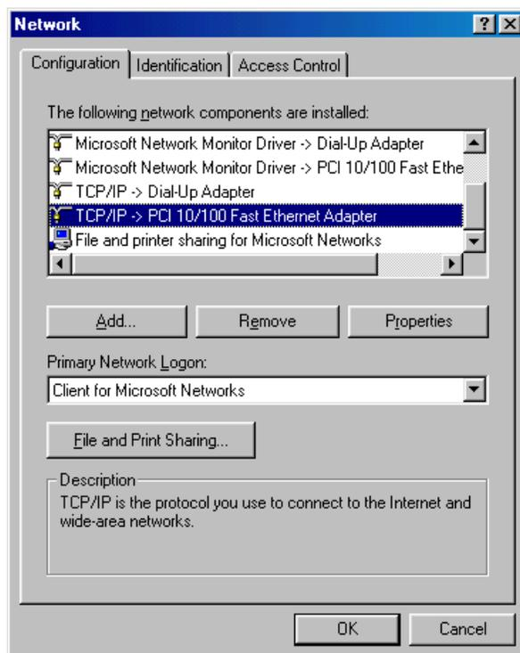
Click the **Properties** button, then choose the **IP Address** tab. Select **Obtain an IP address automatically**.
