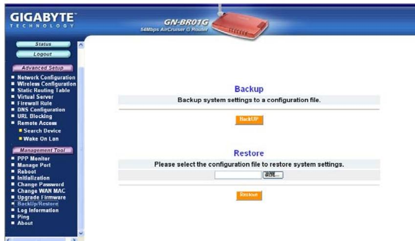
Figure 7-8 – Backup/Restore configurations
