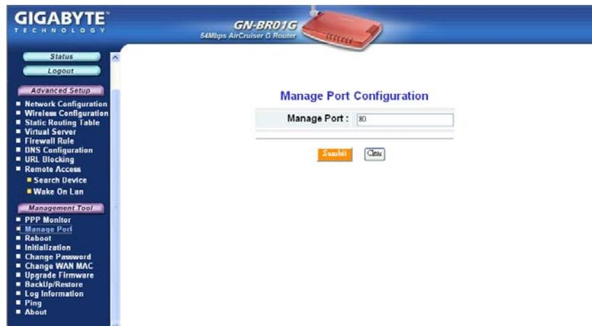
Figure 7-2 – Manage Port Config screen
