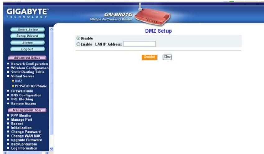
Figure 6-11 – DMZ setup
