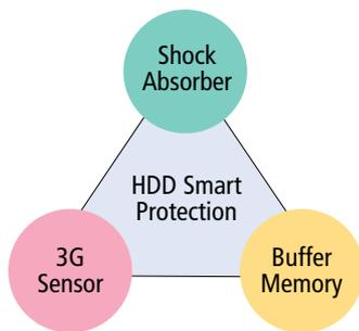
1) Rubber shock absorbers hold the HDD unit in place, helping to prevent external shock from being transmitted when the HVR-DR60 chassis is subject to impact.
