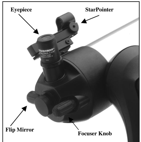
Attach the included accessories (eyepiece and StarPointer finderscope) and remove the front lens cover. Turn-on the Star Pointer by rotating the dial on the side. (For instructions on aligning the Star Pointer see the *Assembly* section of the manual).
