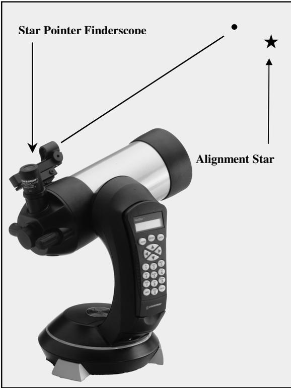
The NexStar will automatically pick an alignment star and slew the telescope close to that star. Once there, the display will ask you to use the arrow buttons to aim the Star Pointer at the star. If the star is not visible (perhaps behind a tree), press UNDO to select a new star. Next, center the star in the eyepiece and press ALIGN. Repeat these steps for the second star alignment. When complete, display will read "Alignment Successful".
