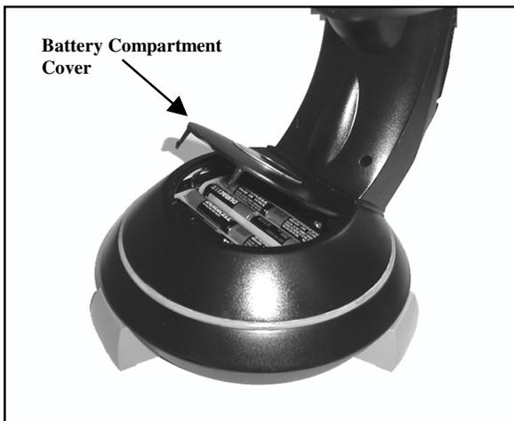
Rotate the tube so it is level with the ground. Lift the battery compartment cover to install batteries. Power the NexStar using the switch next to the 12v outlet at the base of the fork arm.
