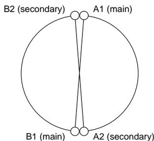
If case of problem with the main heads, for example if only one channel is being recorded and playback cannot be done, you can temporarily switch to the secondary heads so that the playback picture can be viewed. (In case of problem with the main heads, it is recommended to have the unit repaired as soon as possible.)
