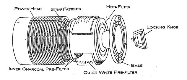
NOTE: The strap fastener should be attached to the inner carbon side of the pre-filter assembly.
