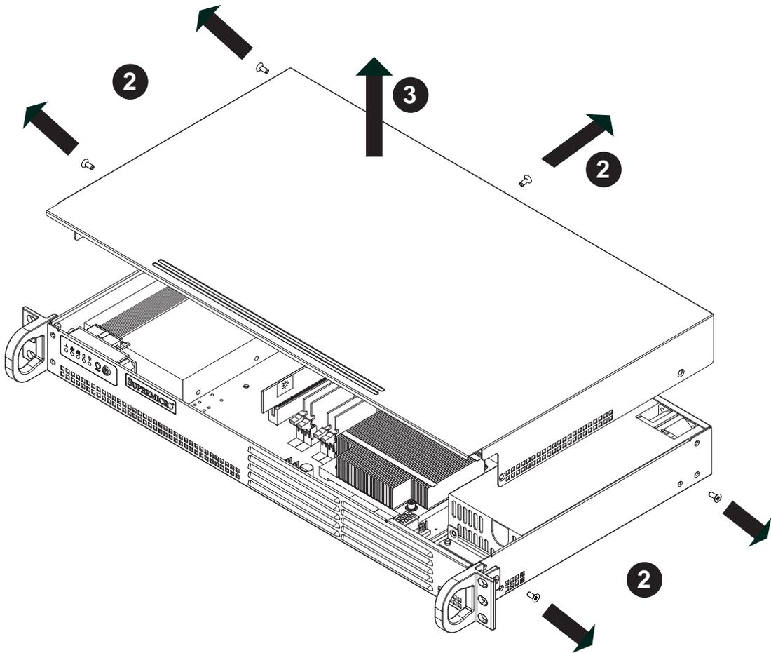
Figure 2-3. Accessing the Inside of the System
