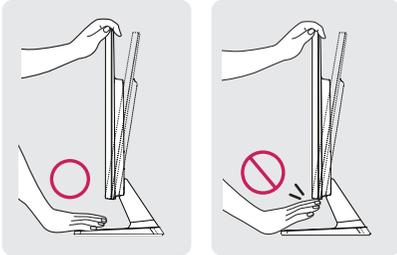
Do not touch or press the screen when adjusting the angle of the monitor.
