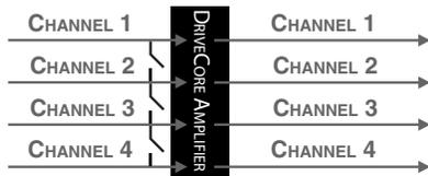
Figure 4.6.1 Four channels with no input routing
