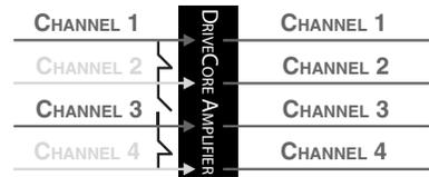
Figure 4.6.3 Two channel to four channel routing
