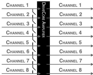
Figure 4.6.2 Eight channels with no input routing
