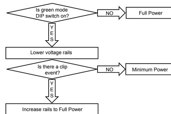
Figure 9.2.1 How Green Power DIP switches work
