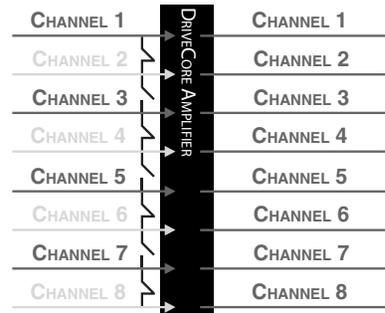
Figure 4.6.5 Four channel to eight channel routing
