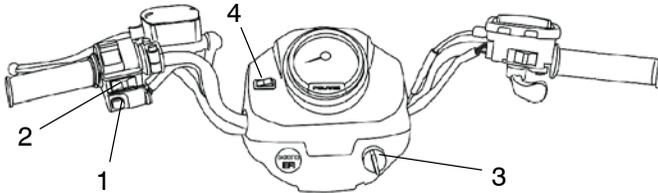
**Mode/Reverse Override Switch (1)** - This vehicle is equipped with a reverse speed limiter system. To gain additional power while backing, depress the override switch.
