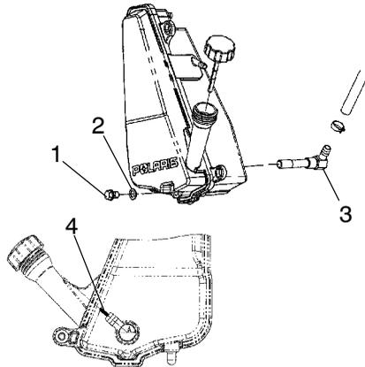
**NOTE:** The fitting threads must be sealed with LOCTITE PST 505 or PTFE seal tape.
