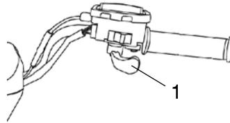
This ATV is equipped with Polaris Electronic Throttle Control (ETC), which is designed to reduce the risk of a frozen or stuck throttle. If the throttle cable should stick in an open position when the operator releases the throttle lever, the engine will stop, and power to the rear wheels will cease.
