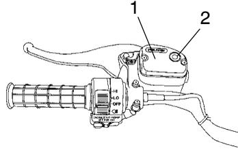
**NOTE:** When checking the fluid level, the ATV must be on level ground with the handlebars straight. If the fluid level is low add DOT 3 brake fluid only. See page 107 for the part numbers of Polaris products.
