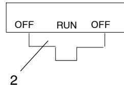
**Main Switch (3)** - To start the engine, slide the stop switch to the center *RUN* position and turn the main key switch clockwise past the *ON* position. Release the key when the engine starts.
