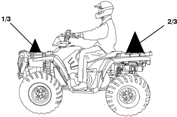
Your ATV has been designed to carry or tow a certain amount of load. Always read and understand the load distribution warning labels on the vehicle, and never exceed the weight capacities outlined in the specifications section of the owner's manual and on the safety decals.
