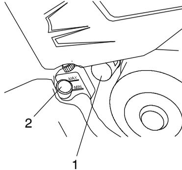
13. Reinstall the drain plug and torque to 14 ft. lbs. (19 Nm).
