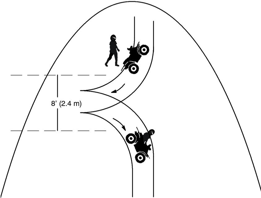
1. Stop and lock the parking brake while keeping body weight uphill.
