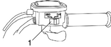
When in AWD, the front gearcase will automatically engage any time the rear wheels lose traction. When the rear wheels regain traction, the front gearcase will automatically disengage.
