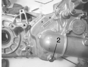
1. Remove the fill plug and the transmission drain plug.
