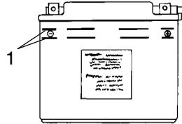
To refill use only distilled water. Tap water contains minerals that are harmful to a battery.
