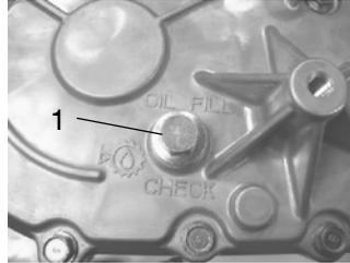
1. Position the ATV on a level surface and remove the fill plug.
