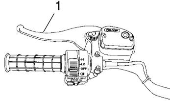
Always test brake lever travel and master cylinder fluid level before riding.
