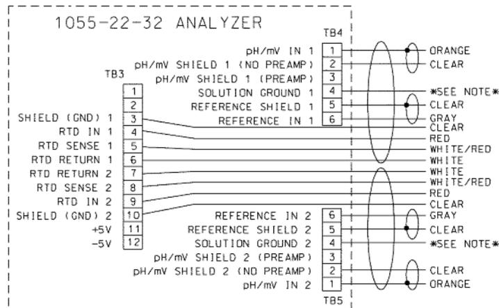
FIGURE 2-14. VP6 3081 & 4081 Wiring
