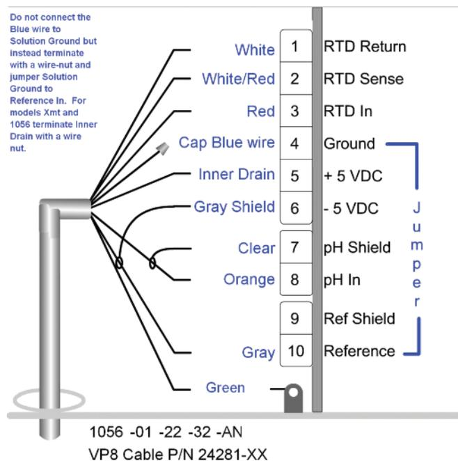
**FIGURE 2-27. 5081 VP8 Wiring.** This is the standard VP8 cable wiring. VP8 cable assembly works both with VP6 and VP8 sensor connector
