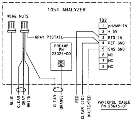
FIGURE 2-18. VP6 1054A/B and 2054 Wiring
