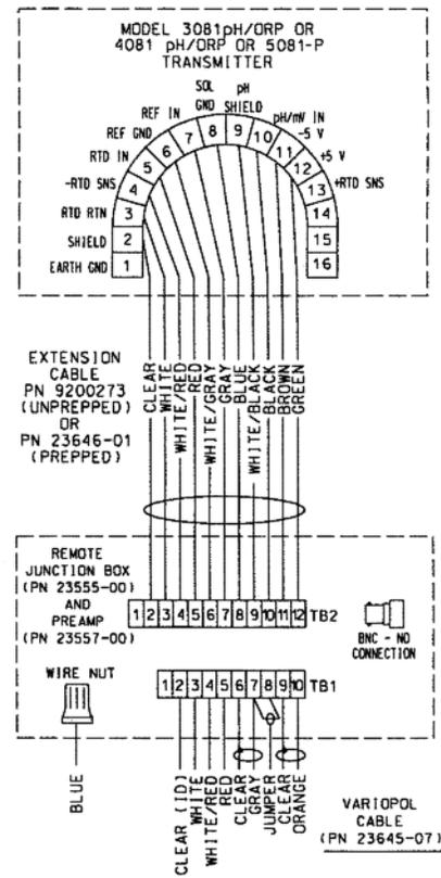
FIGURE 2-17. VP6 1054 Wiring
