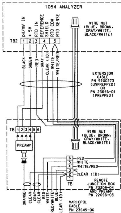
FIGURE 2-20. 1054A/B & 2054 VP6 Wiring through a Remote Junction Box
