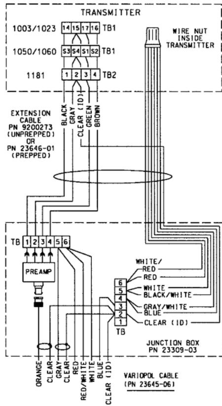
FIGURE 2-12. VP6 2081 Wiring through Remote Junction Box
