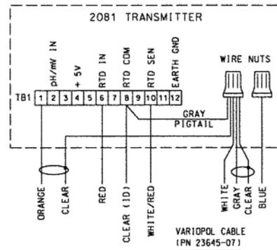
FIGURE 2-11. VP6 1181, 1050/1060, and 1003/1023 Wiring through Remote Junction Box
