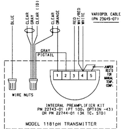
FIGURE 2-8. VP6 54 Wiring through Remote Junction Box
