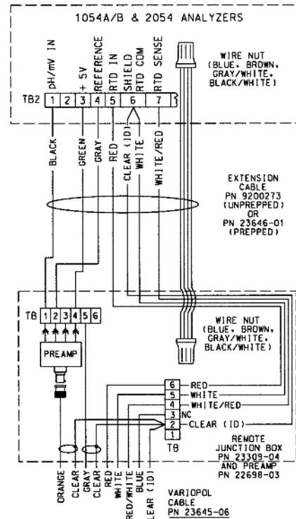
FIGURE 2-21. 1055-22-32 VP6 Wiring through Remote Junction Boxes
