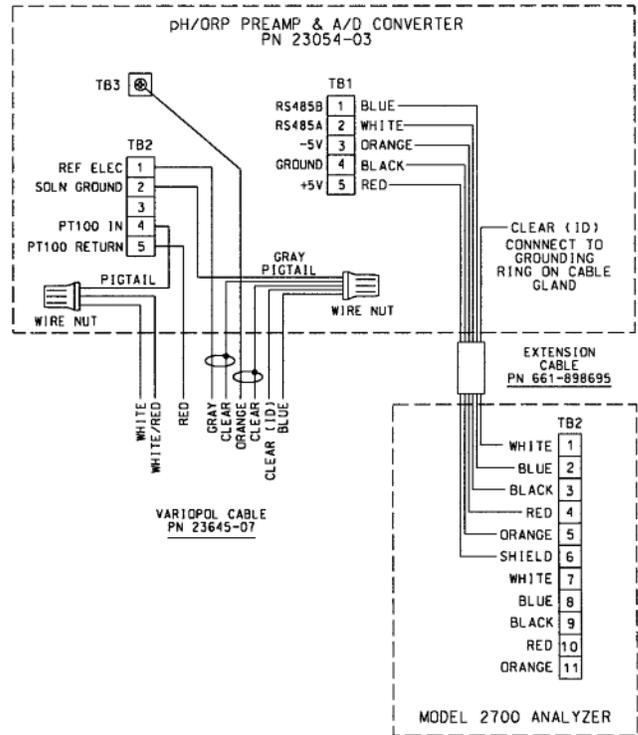
FIGURE 2-23. 54e pH/ORP Wiring. This is the standard VP8 cable wiring. VP8 cable assembly works both with VP6 and VP8 sensor connector
