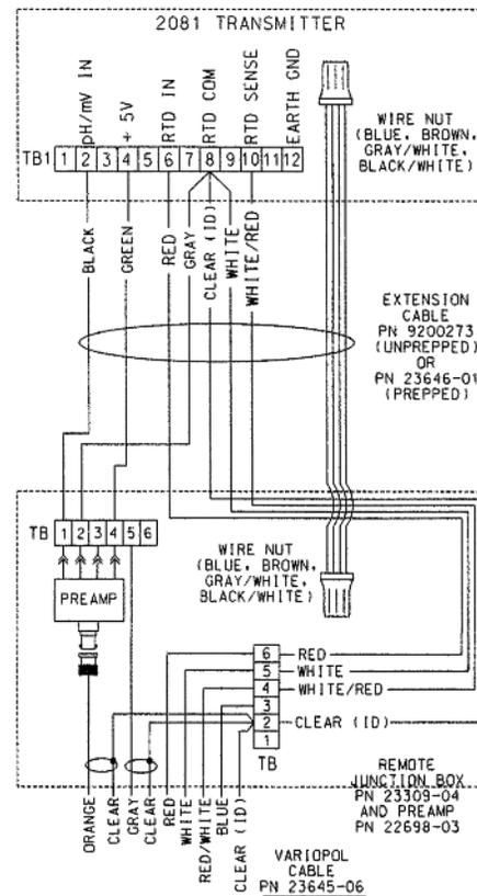
FIGURE 2-13. VP6 1055-22-32 Wiring
