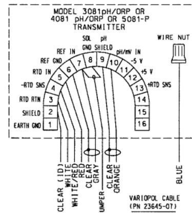
FIGURE 2-15. VP6 81 Wiring through Remote Junction Box
