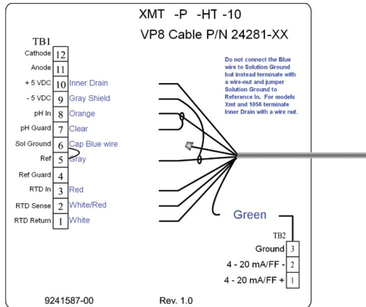
**FIGURE 2-26. 1056 VP8 Wiring.** This is the standard VP8 cable wiring. VP8 cable assembly works both with VP6 and VP8 sensor connector
