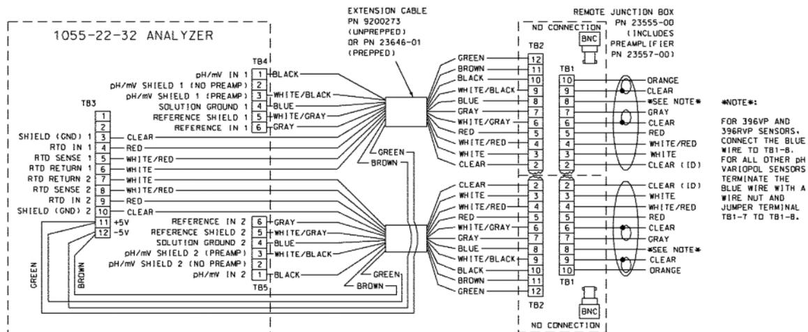
FIGURE 2-22. SCL-(P/Q) Wiring
