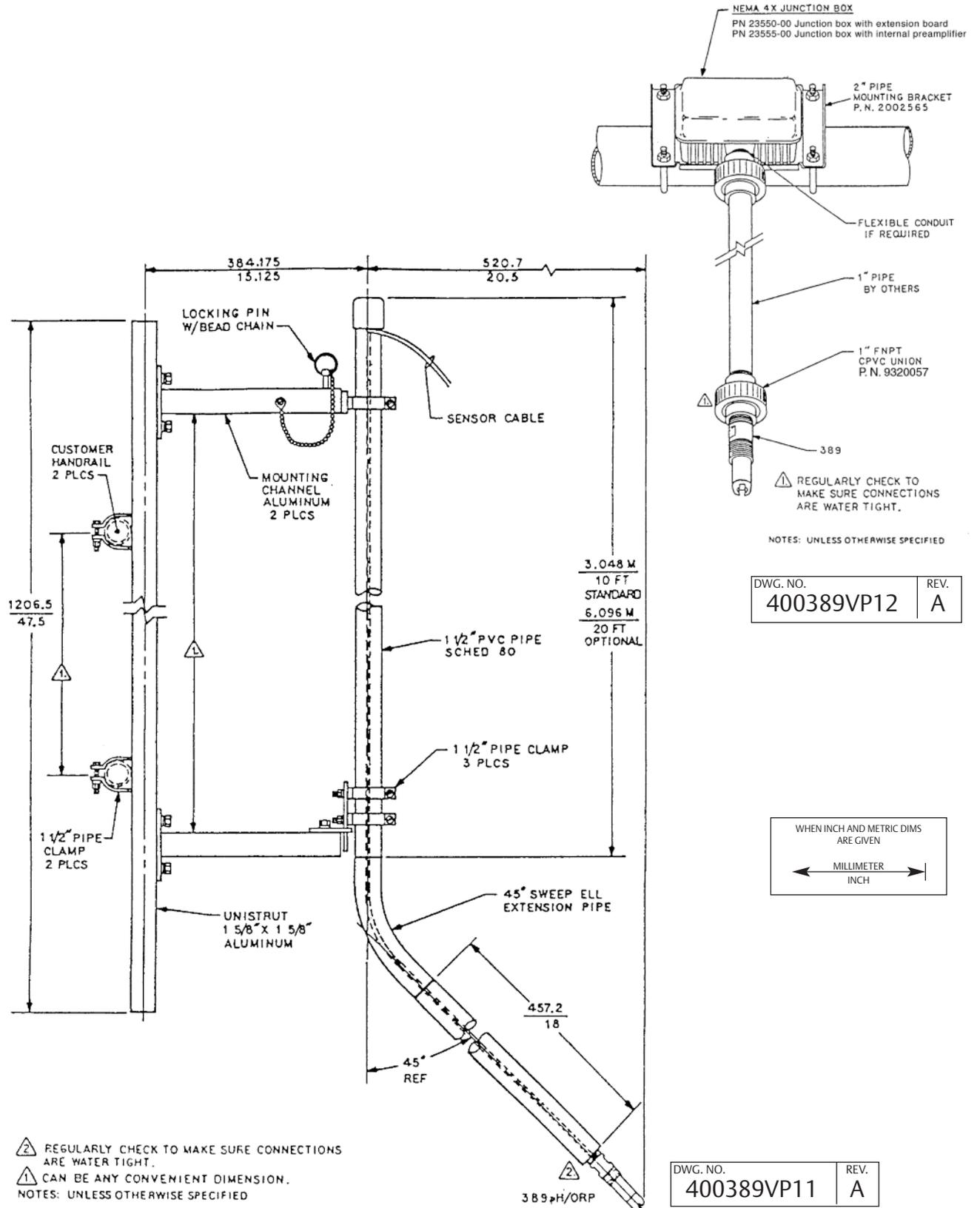
FIGURE 2-3. Flow Through and Insertion Installations
