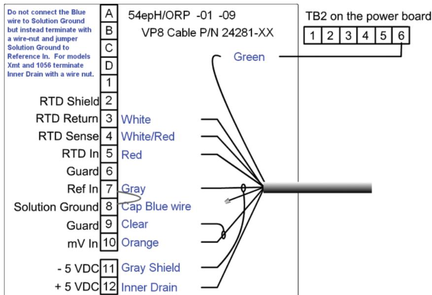
**FIGURE 2-25. Xmt VP8 Wiring.** This is the standard VP8 cable wiring. VP8 cable assembly works both with VP6 and VP8 sensor connector
