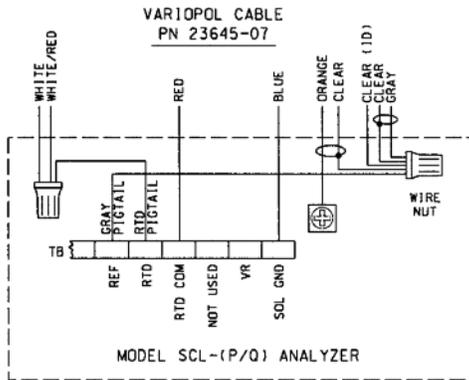
FIGURE 2-23. 2700 Wiring
