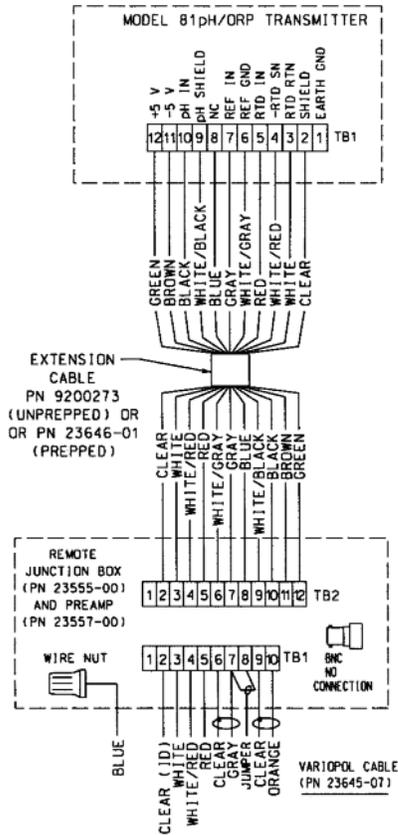
FIGURE 2-16. VP6 3081 & 4081 Wiring through Remote Junction Box
