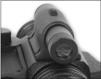
By pressing "SL" button three times you can switch to **Red diode "I"**. **Red diode** represents 100M infra-red illuminator's brightness adjustment mode. Adjustments can be easily observed through the Aries scope while pressing "+" / "-" adjustment buttons.
