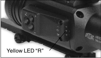
By pressing the SL button twice you switch to a **yellow "R" diode** next to the green one. The **yellow diode** represents the reticle's brightness. Adjustments could be easily seen if you look through the Aries MK6600/6650/7700/7750/8700/8750 while pressing "+" / "-" adjustment buttons.
