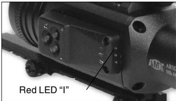
To change the field of coverage from the IR illuminator, focus the beam by turning IR illuminator lens to slightly alter the beam width.
