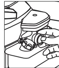
**Step 7** Push the primer ball three times. Wait 3 seconds between each push. **Note:** in cold weather push 5 times.
