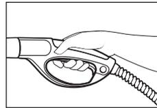
**Step 2** Press trigger to release water pressure.
