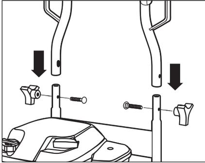
**Step 1** Attach the handle to the frame of the pressure washer. Align holes, insert bolt, and tighten with knob.
