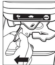
**Step 6** Slide the throttle control to the run position.
