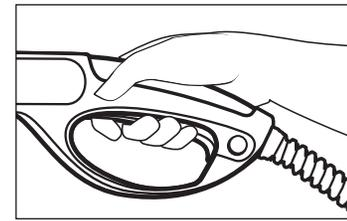
**Step 5** Trigger the gun to eliminate trapped air, wait for a steady flow of water to emerge from the spray nozzle.
