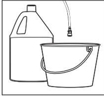
**Step 1** Remove detergent suction tube from container and insert into one gallon of fresh water. Siphon water at low pressure for one minute.
