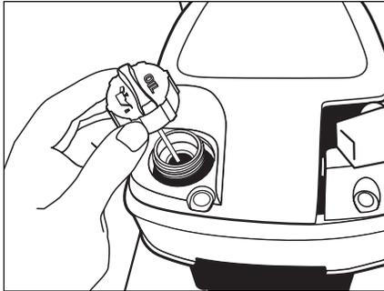
**Step 3** Check oil level. Oil level should always be between the "FULL" and "ADD" marks on the dipstick. Be sure the machine is level when checking the oil level. (Refer to the engine's operating manual for seasonal grades.)
