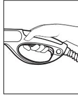
**Step 4** Press trigger to release water pressure.
