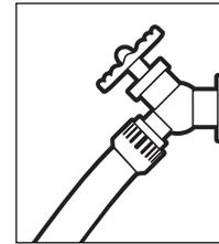
**Step 4** Connect garden hose to the cold water source and turn water on completely.
