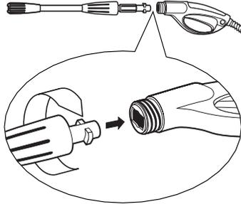
**Step 2** Slide the wand extension into the gun. Turn the wand collar clockwise onto the gun threads until tight.
