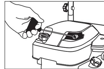
**Step 8** Pull the starter handle. If the engine fails to start after 3 pulls squeeze the trigger gun to release pressure, and repeat step 8.
