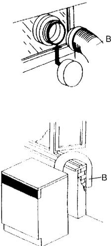
For open window venting it must be possible for the end of the hose to be directed **downwards** to prevent warm, moist air condensing in the room or in the dryer.
