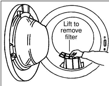
Grip the plastic handle and pull filter upwards (see diagram). The fluff that has collected can now be removed.
