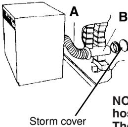
**B** Depending on the frequency of use, it is essential that the areas A and B in the illustrations are checked periodically and any fluff or debris removed.
