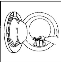
7. When finished, open the door and take out the laundry. Clean and replace the fluff filter.
