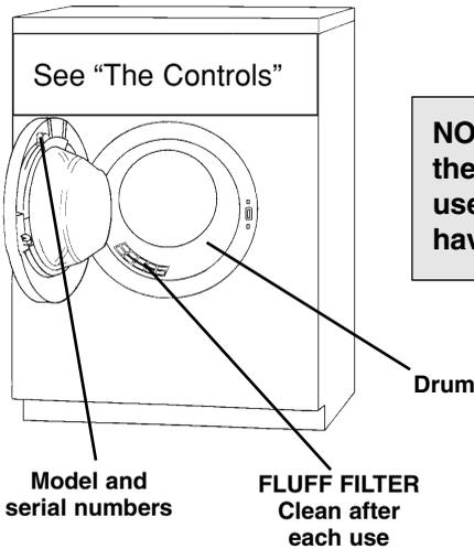
**NOTE:** if your dryer is new wipe out the inside of the drum before you first use it to remove any dust which may have accumulated during transit.
