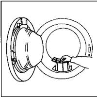
3. Open the door. Check that the fluff filter is clean. Lift filter upwards, clean away any fluff, replace filter correctly.
