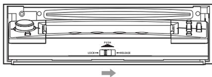
3. Push and slide the DCP upward to remove.
