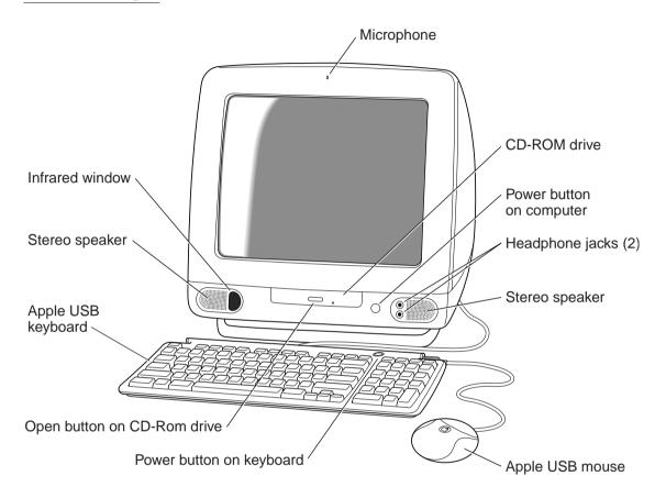
The front of the case is dominated by the 15-inch display. The front also includes, below the display, the following features:
