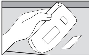
Be careful not to place the fastener strip over the unit's serial number. If the fastener strip is removed, the serial number may be pulled off the unit. Units without serial numbers are not covered under warranty.
