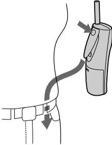
Open the belt clip of the cordless handset by pressing the top of it, and then attach the cordless handset to the belt.
