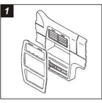
Disconnect the negative battery terminal to prevent an accidental short circuit. Unclip the dash trim bezel. Remove (4) hex-head screws securing the factory head unit and disconnect the wiring.
