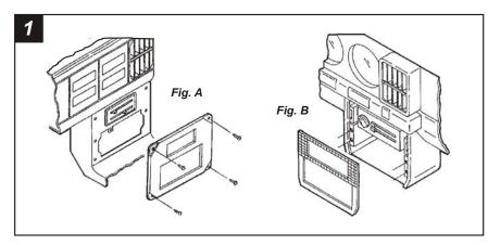
**CAMARO 1982-92, FIREBIRD 1982-84:** Disconnect the negative battery terminal to prevent an accidental short circuit. Remove (4) torx-head screws from the radio trim bezel. Remove (4) hex-head screws securing the factory radio dummy plate and remove the plate. *(see Fig. A)*
