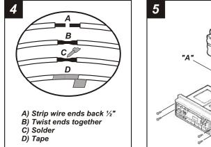
Locate the factory wiring harness in the dash. Metra recommends using the proper mating adaptor and making connections as shown. (Isolate and individually tape off the ends of any unused wires to prevent electrical short circuit).
