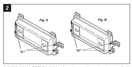
**CAMARO 1985-92, FIREBIRD 1985-92:** Cut and remove all mounting tabs on the **Radio Housing** EXCEPT tabs **"C".** The mounting tabs can be identified by the stamped letter on the back of each tab. (see Fig. A). Skip to the Installation Instructions for ALL VEHICLES on Page #3.
