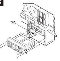
Re-connect the battery terminal and test the unit for proper operation. Screw the *Rear Support* Bullet onto the bolt on the back of the aftermarket head unit ("A"). Mount the radio/kit assembly to the sub-dash with those screws previously removed in step #1.
