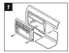
Disconnect the negative battery terminal to prevent an accidental short circuit. Remove the ashtray and (1) Phillips screw exposed in the ashtray cavity. Open the glove box and remove (2) Phillips screws exposed on the right edge of the radio trim bezel. Remove the radio trim bezel and disconnect the wiring.
