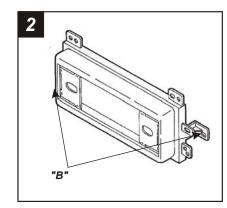
Cut and remove all mounting tabs on the **Radio Housing** EXCEPT tabs **"B"**. The mounting tabs can be identified by the stamped letter on the back of each tab. *Skip to the Installation Instructions for ALL VEHICLES on Page* #3.
