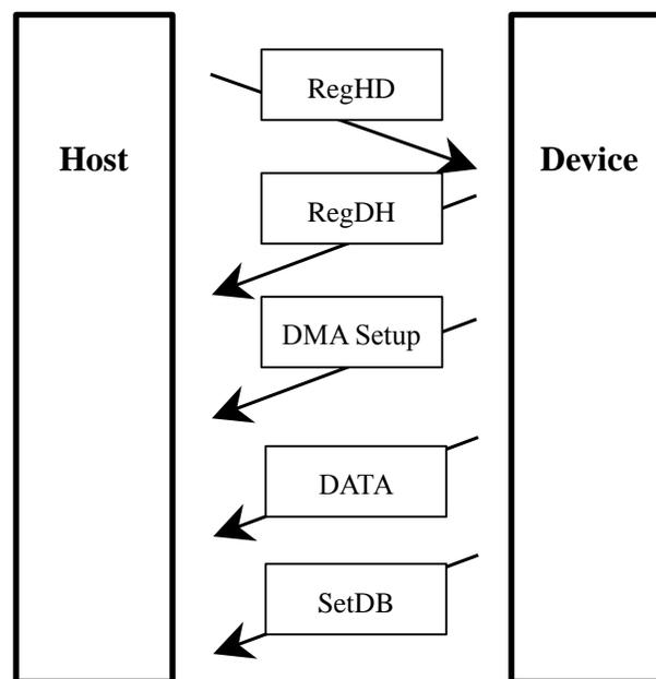
Figure 5.18 READ FP DMA QUEUED command protocol
