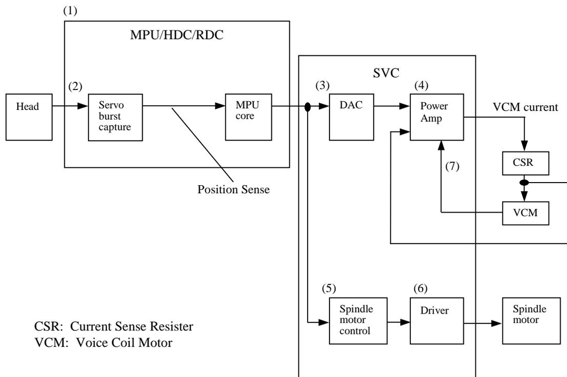
**Figure 4.6 Block diagram of servo control circuit**
