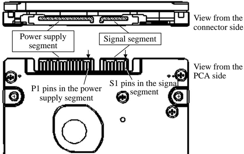
**Figure 3.9 Power supply pins (CN1)**
