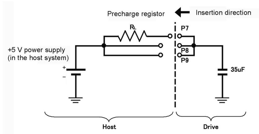
It is necessary to choose pre-charge resistor  $R_L$  value, which is in permissible range of +5V power supply specification at the host system.
