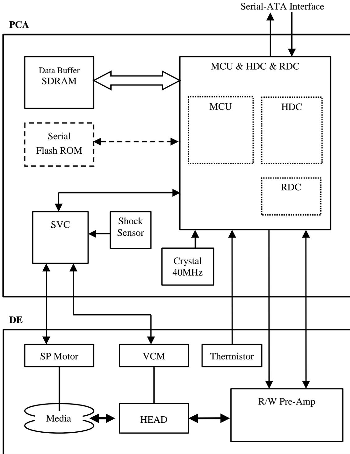
Figure 4.2 Circuit configuration
