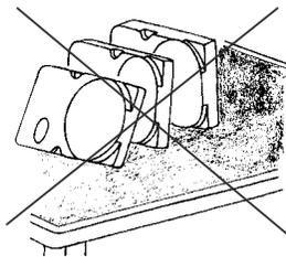
Do not place HDD vertically to avoid falling down.
