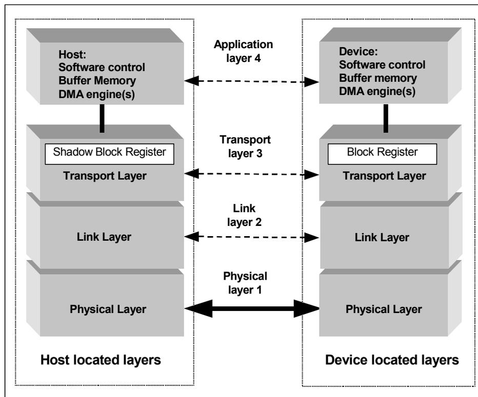
Figure 5.3 Conceptual diagram of communication layers
