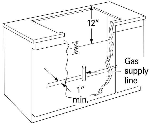
**Note:** Reference Instructions, GE Monogram 30" Stainless Steel Cooktop Installation, packed with product, for complete details. The house gas supply should be at least 1" from the back wall. The electrical outlet should be 12" below the countertop and within reach of the 4 ft. power cord.
