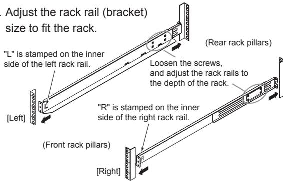
2. Attach the rack rails (brackets) to the rack. The size of the ETERNUS DX60/DX80 is 2U.
