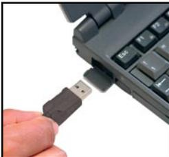
3. Plug the cable into the port (USB or LAN) on your computer.
