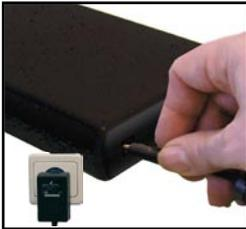
2. Insert the power cord into the Freecom Network Drive XS and plug the power supply into the socket.
