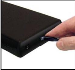
1. Plug the cable (USB or LAN) into the Freecom Network Drive XS.
